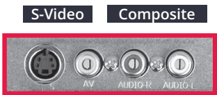
S-Video (YCbCr / AVS) Input Connector Composite Video Connector
