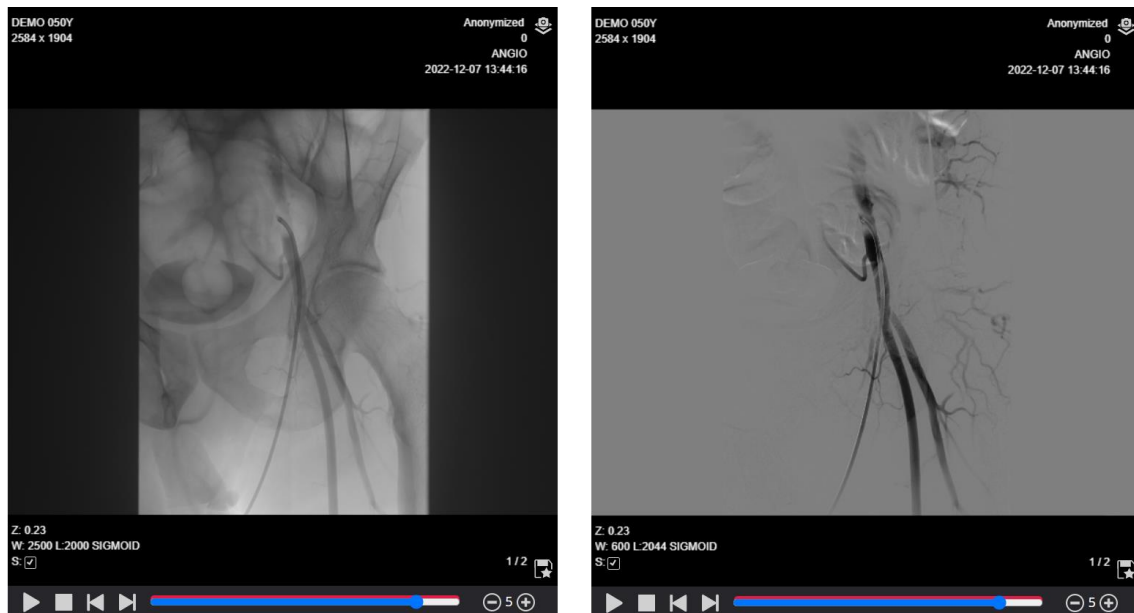
Figure 54. The angiography multiframe image without (on the left), and after the mask subtraction (on the right)
